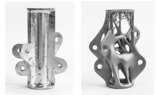
Fabricated design optimised for DMLS. (Arup Amsterdam).
