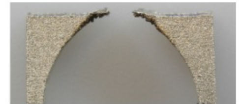
Over sized holes or unsupported sections can fail.
